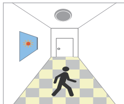
With sufficient daylight, even when motion detected, light remains OFF.
